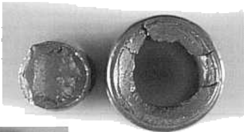
Fig. 3 — Cracks & burst visible on point end of bolts.
