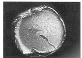
Fig. 6 — Fracture located on underside of head on failed hex bolt.
