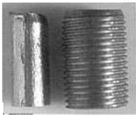
Fig. 4 — Bottom & side views of core material (l) that fell out of the threaded portion (r) of the bad bolt after sectioning.
