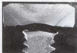
Fig. 8 — Wing-like indications in the bolt head.
